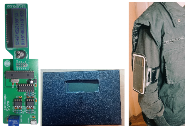
Picture 3 – Personal Magnetic Field Dosimeter: Structure, Appearance, and Usage (10)
